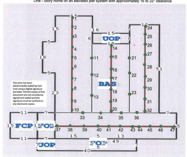
Push Pier Model 300: Interior Pier: Polyurethane 700: Push Pier Model 250: Low Profile Bracket: Polyurethane 430: Helical Pier: Porch Bracket: **Exsisting Beams** Crawl Space Pier: 4x6 Wood Beam: Floor Joist:
