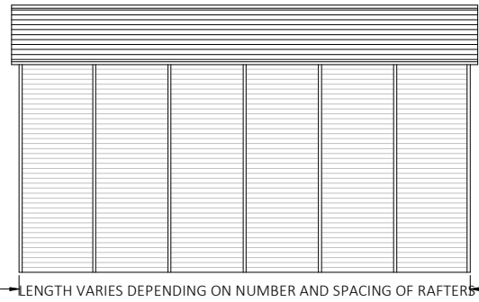
TYPICAL SIDE ELEVATION - HORIZONTAL ROOF
