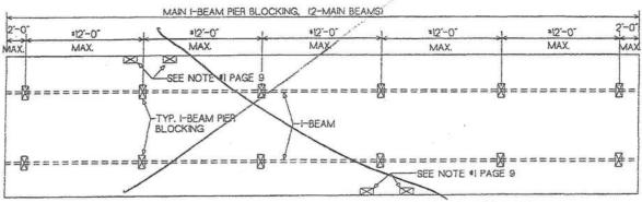
\*MAXIMUM SPACING OF PIERS IS NOT TO EXCEED 8 FEET FOR 8 INCH I-BEAM, 10 FEET FOR 10 INCH I-BEAM AND 12 FEET FOR 12 INCH I-BEAM.
