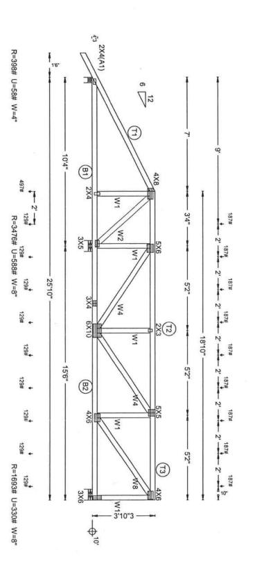
LEFT RAKE = 1'8"2 LEFT JIG = 7'11"14 TAG = T11 PLT. TYP.-WAVE
