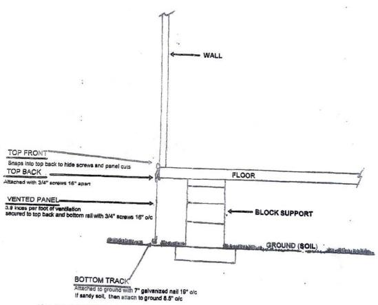
\*ALL PANELS ARE ACCESSIBLE BY REMOVING TOP FRONT AND PULLING UP ON PANEL
