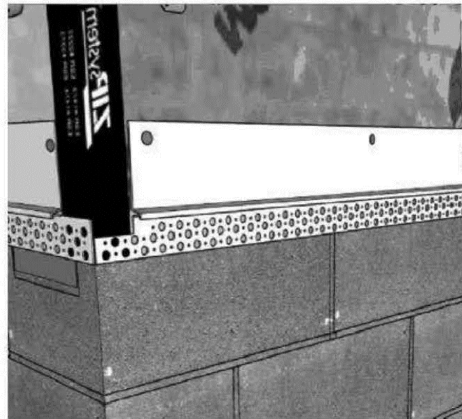
2 MID-WALL STARTER STRIP: NOTCH CORNER TO ACCEPT TRIM BEFORE INSTALLING. NOTCH TO EXTEND MIN. 3/4" BELOW TOP OF CMU
