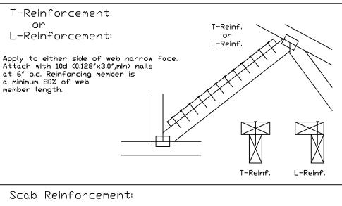
Apply scab(s) to wide face of web. No more than (1) scab per face. Attach with 10d (0.128"x3.0",min) nalls at 6" o.c. Reinforcing member is a minimum 80% of web member length.
