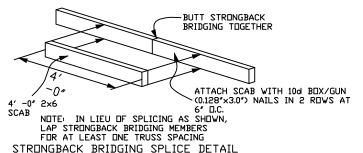
NOTE: Details 1 and 2 are the preferred attachment methods ATTACH STRONGBACK TO WEB W/ (3) 10d COMMON-(0.148"x3") NAILS DR (4) 10d BDX/GUN 03128"x3.0") NAILS
