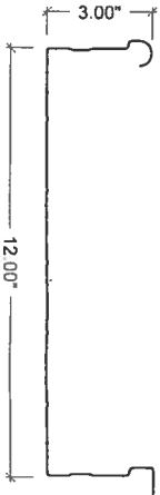
12" WIDE x 3" RISER INTERLOCKING ROOF PANEL SCALE: 2" = 1'-0"
