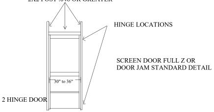
EACH DOOR IS SCREWED INTO UPRIGHTS WITH #10 1" 6" FROM ENDS 24" O.C.
