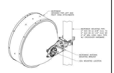
MICROWAVE & ODU MOUNTING DETAIL SCALE: NOT TO SCALE
