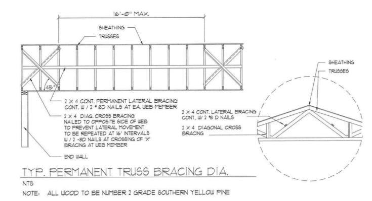
Truss Bracing DETAILS
