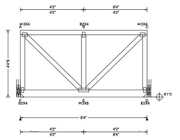
Loading Criteria (psf) TCLL: 20.00 TCDL: 10.00 BCLL: 0.00 BCDL: 10.00 Des Ld: 40.00 NCBCLL: 10.00 Soffit: 2.00 Load Duration: 1.25 Spacing: 24.0 "
