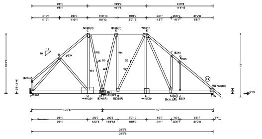
Loading Criteria (psf) TCLL: 20.00 TCDL: 10.00 BCII: 0.00 BCDL: 10.00 Des Ld: 40.00 NCBCLL: 0.00 Soffit: 2.00 Load Duration: 1.25 Spacing: 24.0 "
