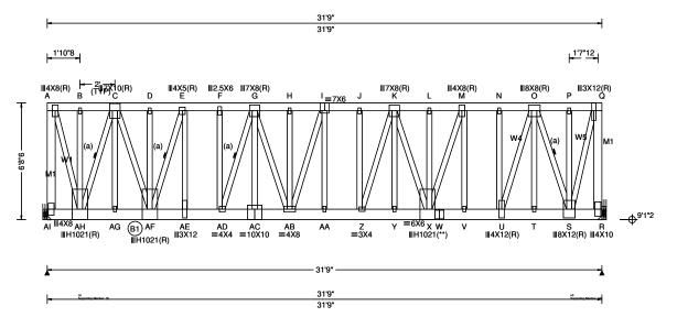
Loading Criteria (psf) TCLL: 20.00 TCDL: 10.00 BCII: 0.00 BCDL: 10.00 Des Ld: 40.00 NCBCLL: 10.00 Soffit: 2.00 Load Duration: 1.25 Spacing: 24.0 "
