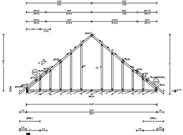
Loading Criteria (psf) TCLL: 20.00 TCDL: 10.00 BCLL: 0.00 BCDL: 10.00 Des Ld: 40.00 NCBCLL: 10.00 Soffit: 2.00 Load Duration: 1.25 Spacing: 24.0 "
