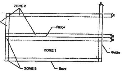
Note: Dimension (a) is defined as 10% of the minimum width of the building or 40% of the mean height of the root, whichever is smaller, however, (a) cennot be less than either 4% of the minimum width of the building or 3 feet.
