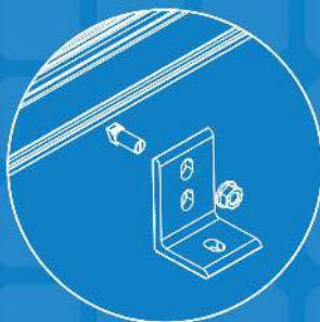
INTEGRATED BONDING MICROINVERTER MOUNT w/ WIRE MANAGEMENT
