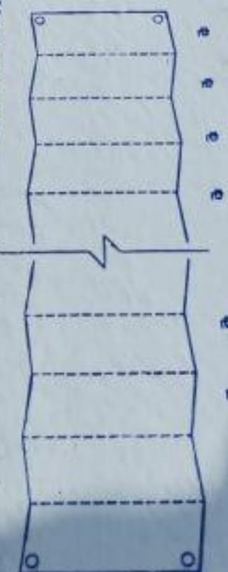
If factory tabs are run **perpendicular to the board**, a fastener in each corner is required. (See drawing B)
