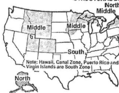
DESIGN ROOF LOAD ZONE MAP
