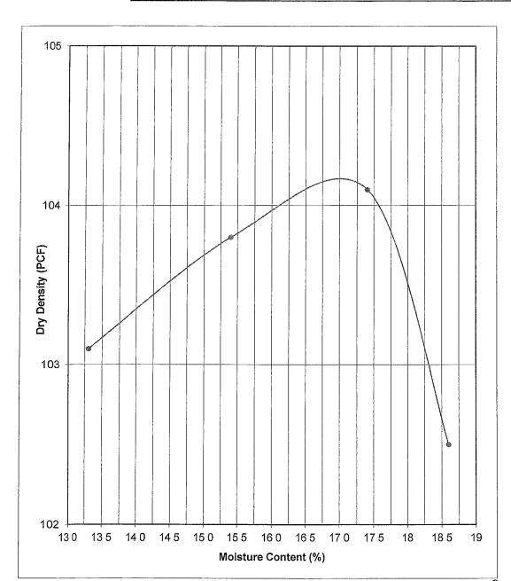
PROCTOR DATA Proctor No.. 1 Modified Proctor 1 (ASTM D-1557) Standard Proctor (ASTM D-698) Maximum Dry Dens Pcf: 104 0 Optimum Moisture Percent: 170 Total -200 (%): 7 9 LL NA NP
