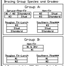
1x4 Braces shall be SRB (Stress-Rated Board) \*\*For 1x4 So. Pine use only Industrial 55 or Industrial 45 Stress-Rated Boards, Group B values may be used with these grades.
