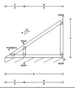
▲ Maximum Reactions (lbs), or \*=PLF Gravity Non-Gravity Loc R+ /Rw /U /RL D\* 84 /-/56 /15 Wind reactions based on MWFRS D Brg Width = 72.0 Min Req = -Bearing A is a rigid surface. Members not listed have forces less than 375#
