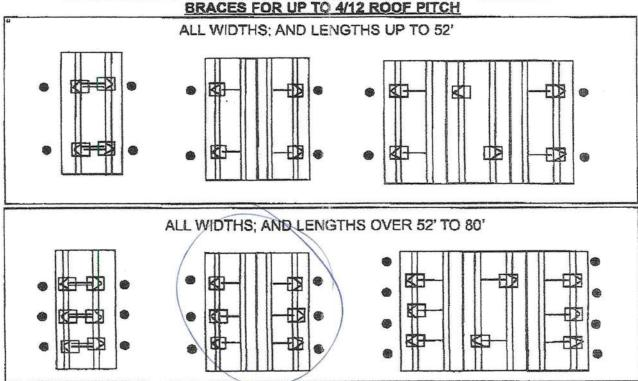
HOMES WITH 5/12 ROOF PITCH REQUIRE: PER FLORIDA REGULATIONS 6 systems for home lengths up to 52' and 8 systems for homes over 52' and up 80'. One stabilizer plate and frame tie required at each lateral bracing system.
