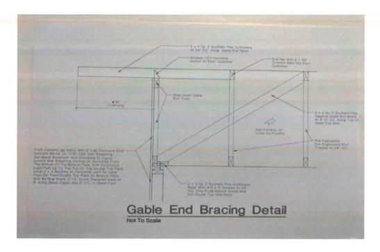
**ROOF FRAMING:** Provide Pre-Fabricated, Pre-Engineered Roof Trusses at 24" O.C. Install Simpson H2A Hurricane Anchors at each truss bearing location as determined by the truss engineering. Install Simpson H10 Hurricane Anchors at each truss bearing location for Uplift Loads greater than 600# and less than 1,100#.
