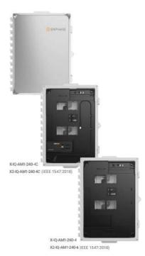
The IQ Combiner 4/4C with IQ Gateway and integrated LTE-M1 cell modem (included only with IQ Combiner 4C) consolidates interconnection equipment into a single enclosure. It streamlines IQ Microinverters and storage installations by providing a consistent, pre-wired sclution for residential applications. It offers up to four 2-pole input circuits and Eaton BR series busbar assembly.
