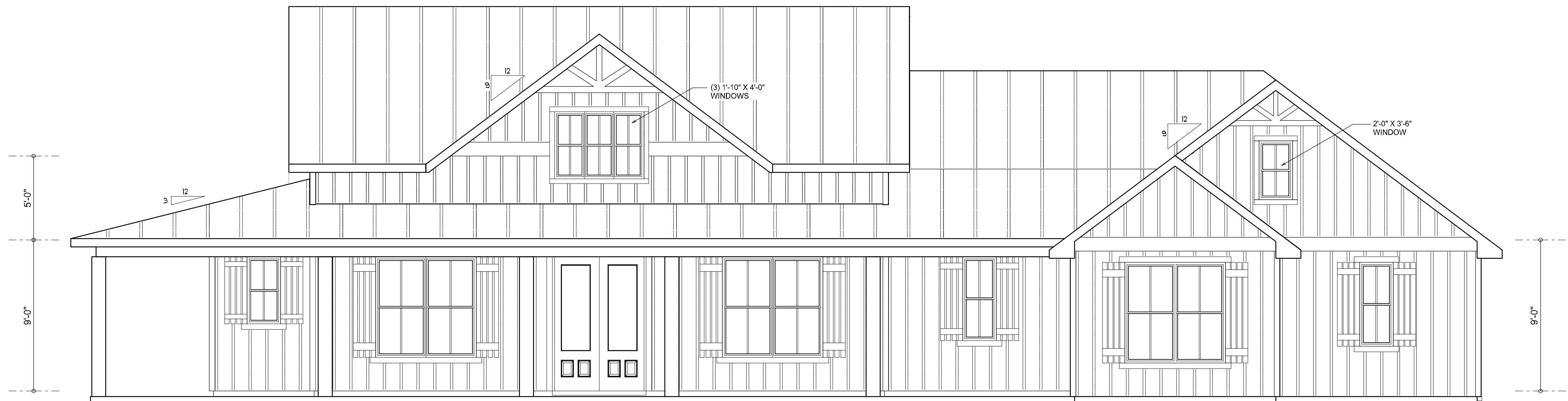
FRONT ELEVATION SCALE: 1/4" = 1'-0"
