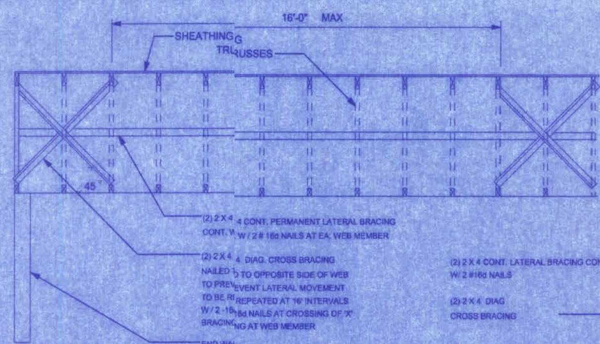
NOTE: ALL WOOD TO BE NUMBER 2 GRADE SOUTHERN YELLOW PINE TYPICAL PERMANENT TRUSS BRACING DIAGRAM NTS
