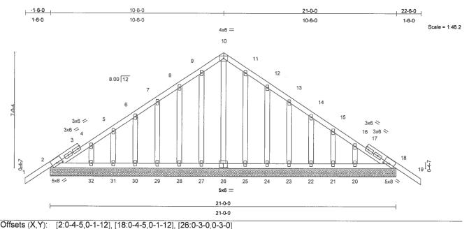
Plate Offsets (X,Y): LOADING (psf) 2-0-0 **SPACING** CSI DEFL I/defl L/d **PLATES** (loc) GRIP in **TCLL** 20.0 Plates Increase 1.25 TC 0.16 Vert(LL) -0.01 19 n/r 120 MT20 244/190 TCDL 7.0 Lumber Increase 1.25 BC 0.04 Vert(TL) -0.01 19 n/r 90 **BCLL** 10.0 Rep Stress Incr NO WB 0.11 Horz(TL) 0.01 18 n/a n/a **BCDL** 5.0 Code FBC2004/TPI2002
