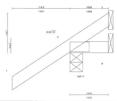
Plate Offsets (X,Y): [2:0-3-9,0-1-8] **SPACING** 2-0-0 LOADING (psf) CSI **DEFL** L/d **PLATES** GRIP in (loc) I/defl **TCLL** 20.0 Plates Increase 1,25 TC 0.16 Vert(LL) -0.00 2 >999 360 MT20 244/190 **TCDL** BC 7.0 1.25 0.01 2 240 Lumber Increase Vert(TL) -0.00 >999 **BCLL** 10.0 \* Rep Stress Incr YES WB 0.00 Horz(TL) 0.00 3 n/a n/a **BCDL** 5.0 Code FBC2004/TPI2002 (Matrix) Weight: 6 lb
