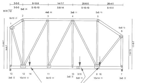
Beam to Truss connection to be specified by the Architect/Engineer of Record.
