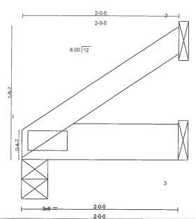
LOADING (psf) **SPACING** 2-0-0 CSI **TCLL** 20.0 Plates Increase 1.25 TC 0.05 **TCDL** 7.0 Lumber Increase 1.25 BC 0.06 **BCLL** 10.0 Rep Stress Incr NO WB 0.00 **BCDL** Code FBC2004/TPI2002 5.0 (Matrix)
