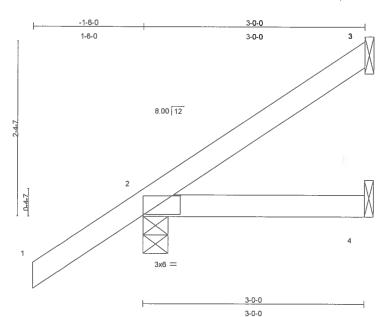
Plate Offsets (X,Y): [2:0-3-9,0-1-8] LOADING (psf) **SPACING** 2-0-0 CSI DEFL I/defl L/d **PLATES GRIP** in (loc) **TCLL** 20.0 Plates Increase 1.25 TC 0.180.01 >999 360 Vert(LL) 2-4 MT20 244/190 TCDL 7.0 Lumber Increase 1.25 BC 0.08 Vert(TL) -0.01 2-4 >999 240 **BCLL** 10.0 Rep Stress Incr WB YES 0.00 Horz(TL) -0.00 3 n/a n/a BCDL 5.0 Code FBC2004/TPI2002 (Matrix) Weight: 13 lb
