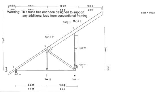
Plate Offsets (X,Y): [2:0-3-9,0-1-8], [4:0-5-11,Edge] LOADING (psf) SPACING 2-0-0 CSI DEFL (loc) I/defl L/d **PLATES GRIP TCLL** 20.0 Plates Increase 1.25 TC 0.48 Vert(LL) -0.03 2-7 >999 360 MT20 244/190 TCDL 7.0 Lumber Increase 1.25 BC 0.20 Vert(TL) -0.072-7 >999 240 **BCLL** 10.0 Rep Stress Incr YES **WB** 0.29 0.01 8 Horz(TL) n/a n/a BCDL 5.0 Code FBC2004/TPI2002 (Matrix) Weight: 121 lb
