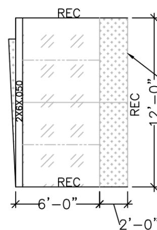
WINDBREAKER GLASS WINDOW AND FOAM PANEL KNEE WALL INSERTS (TYP)
