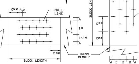
LOAD APPLIED PERPENDICULAR TO GRAIN
