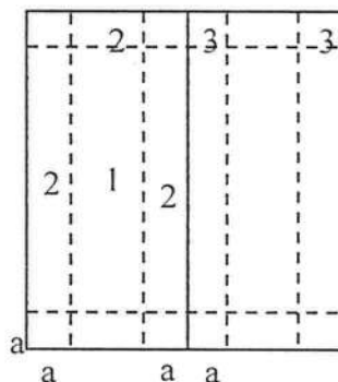
Figure 6-5 - External Pressure Coefficients, G C_p Loads on Components and Cladding for Buildings w/ H_t \leq 60 ft
