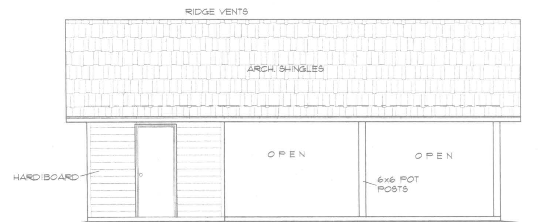
SHELTER LEFT ELEVATION SCALE: 1/4 IN. = 1 FT.
