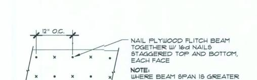
PLYWOOD FLITCH BEAM DETAIL NOT TO SCALE
