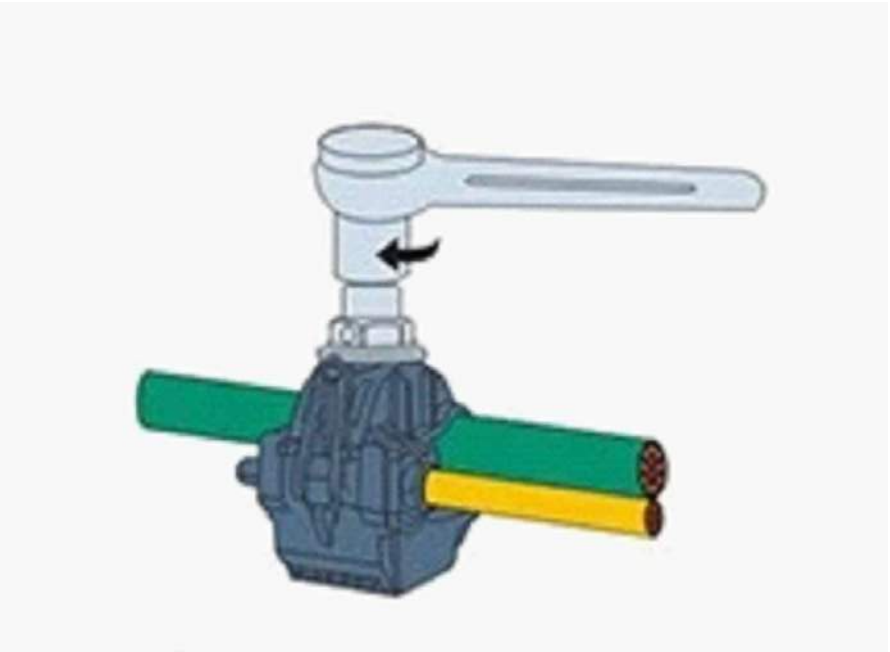
MAKE MODEL VOLTAGE RATING CONDUCTOR RANGE MAIN CONDUCTOR RANGE TAP ILSCO IPC 4006 600 V 4/0-4 AWG 6-14 AWG ILSCO IPC 4020 600 V 4/0-2 AWG 2/0-6 AWG
