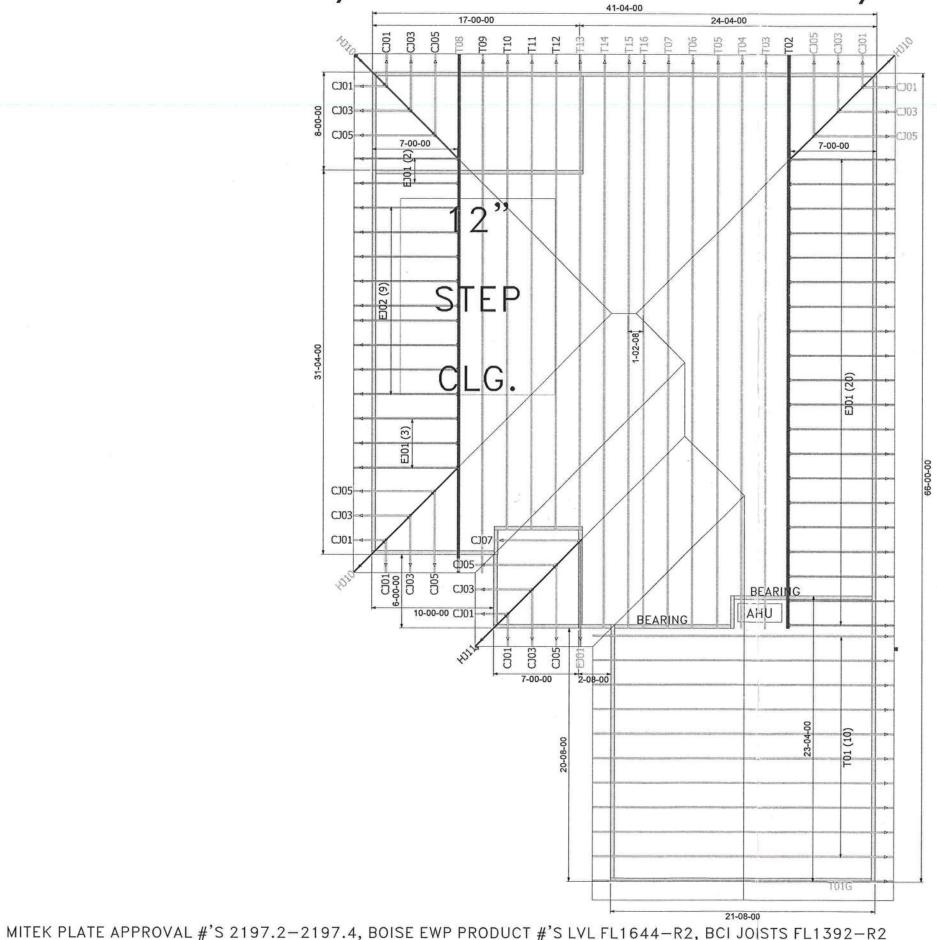
THE ARROW HEAD AT THE END OF THE TRUSS ON THE TRUSS PLACEMENT PLAN (LAYOUT) CORRESPONDS WITH THE LEFT SIDE OF THE INDIVIDUAL TRUSS DRAWING, USE THIS AS AN ORIENTATION GUIDE WHEN SETTING THE TRUSSES ON THE STRUCTURE.
