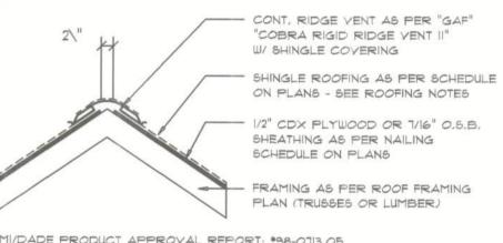
SCHEDULE ON PLANS FRAMING AS PER ROOF FRAMING PLAN (TRUSSES OR LUMBER)
