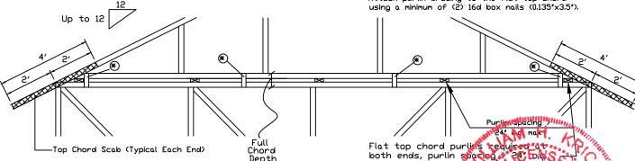
Depth Note: If purlins or sheathing are not specified on the flat top of the sage truss, purlins must be installed at 24" o.c. max. and use Detail A.
