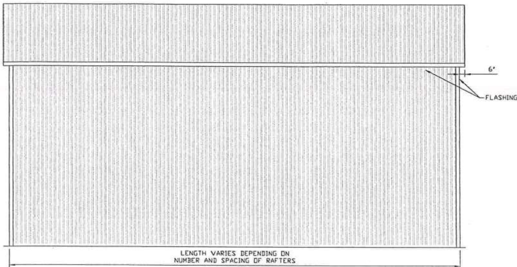
TYPICAL SIDE ELEVATION VERTICAL ROOF/SIDING SCALE: 1/8" = 1'-0"
