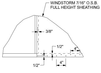
DOUBLE NAIL EDGE SPACING TOP AND BOTTOM PLATE
