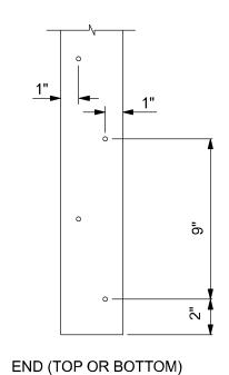
GIRDER COLUMN DETAIL SCALE: 1/2" = 1'-0"
