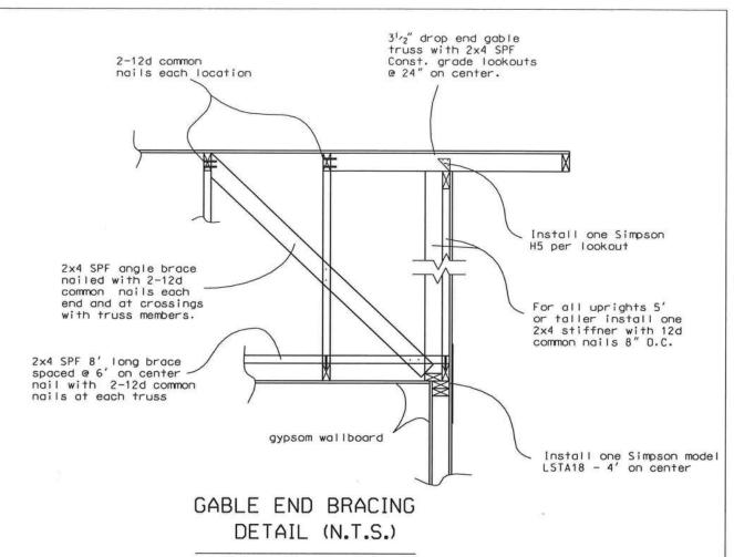
NOTE: Gable end trusses shall be dropped  $3^{1}_{2}$ " for construction of lookouts & overhang.
