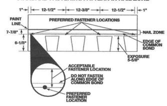
3) Mansard Fastening Pattern. (For use on decks with slopes greater than 21 in. per foot.) One fastener 1 in. from each end and one fastener 8-1/2 in. from each end and one fastener 16 in. from each end for a total of 6 fasteners per shingle. (See Mansard and High Wind Fastening Pattern illustrated below.)
