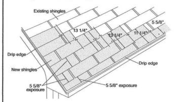
Second and Succeeding Courses: Remove 10-3/8 in. from the rake end of the first shingle in the second course, and continue with full width shingles for the remainder of the course, placing the top edge of each new shingle against the butt edge of the old shingle in the course above. This method should create an exposure of 5-5/8 in. after the first course. When beginning the succeeding courses continue to follow the Heritage application instructions. (See section 5).
