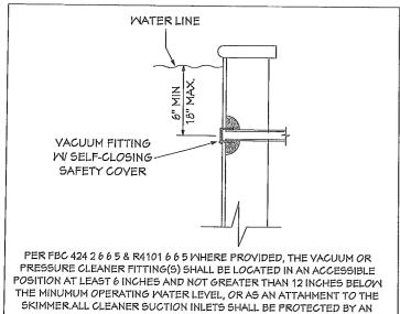
APPROVED, PERMANENTLY INSTALLED, SELF CLOSING FLAPPER
