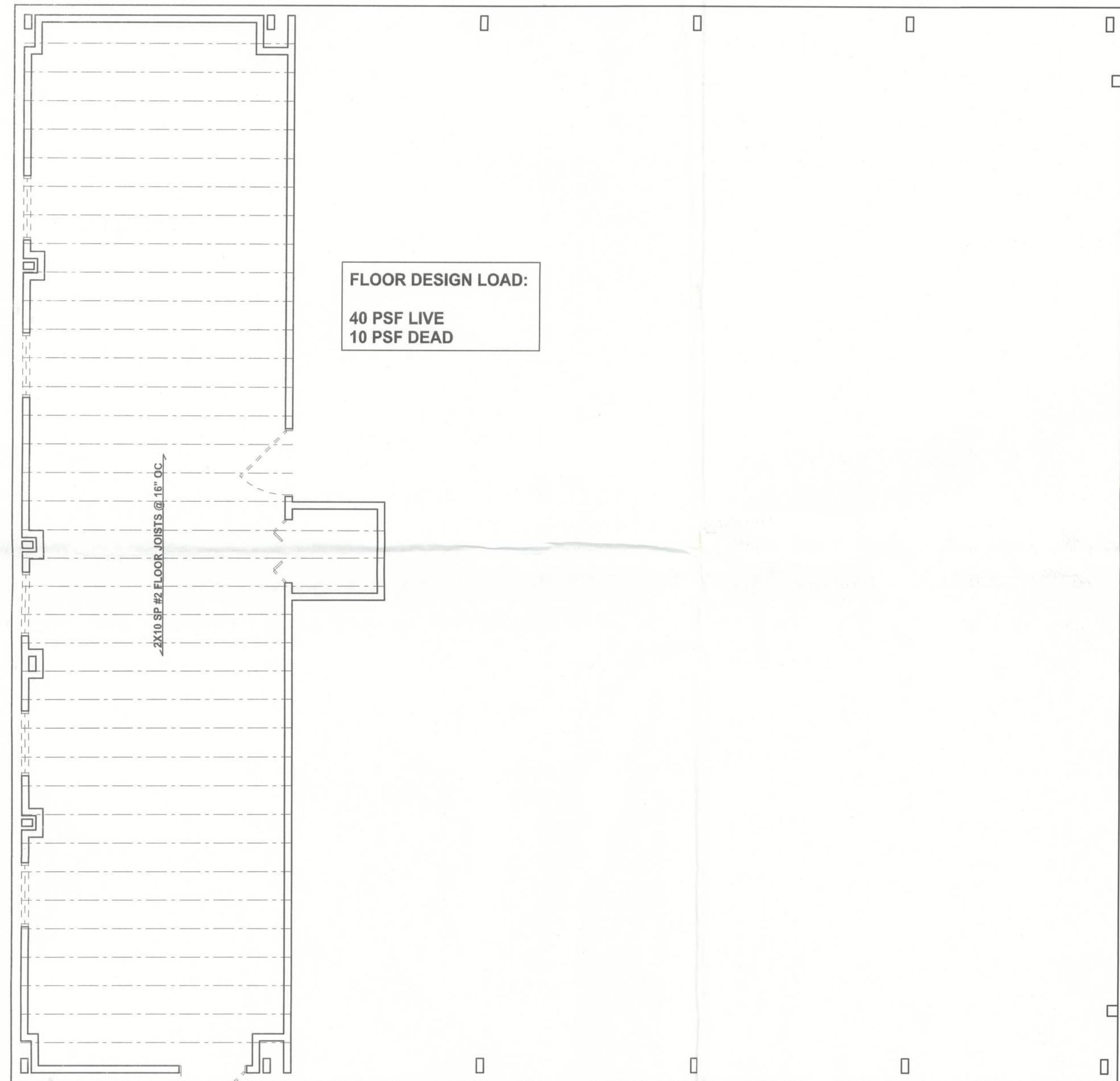
CEILING FRAMING PLAN SCALE: 1/4" = 1'-0"
