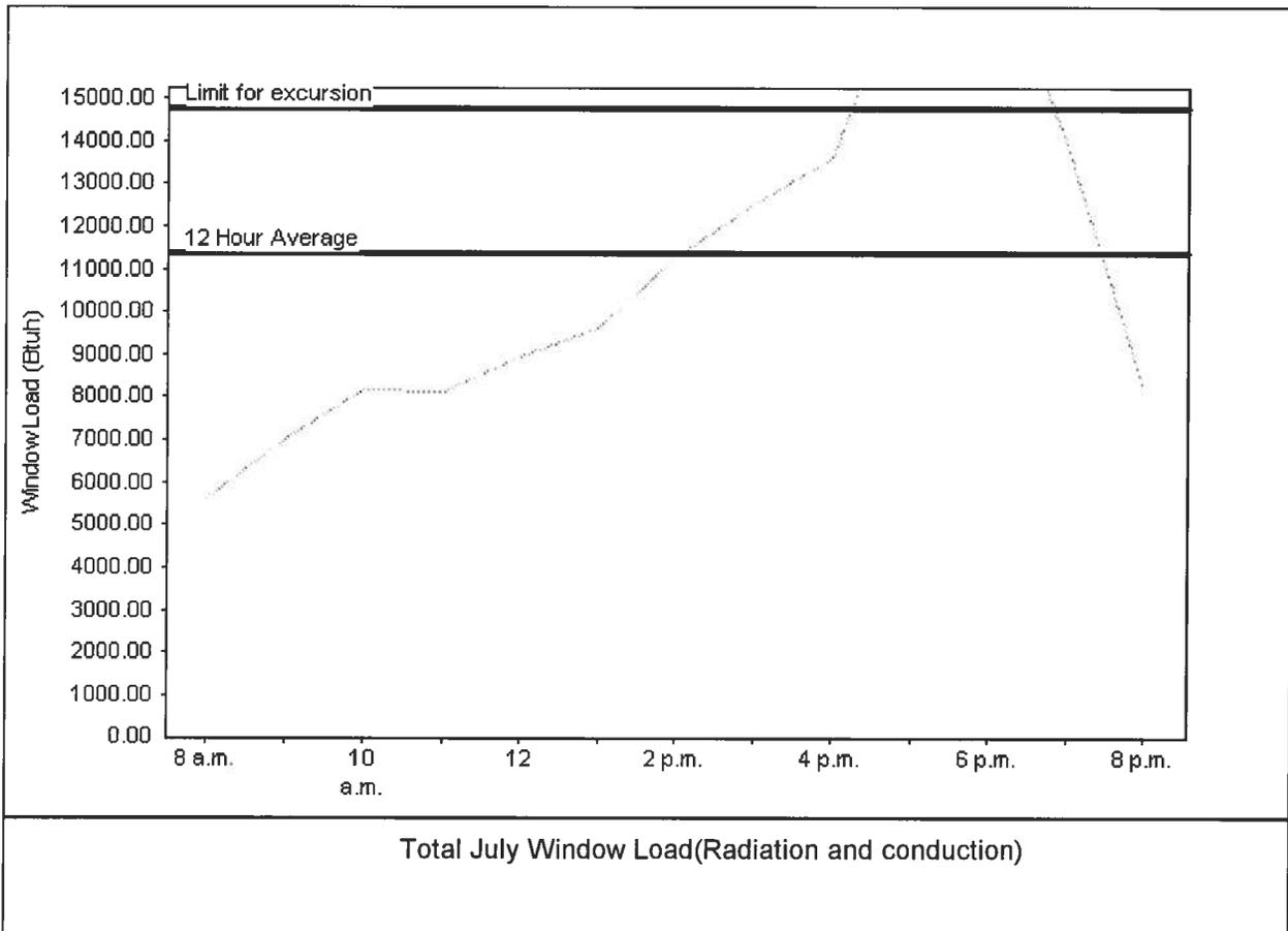
Total July Window Load(Radiation and conduction)
