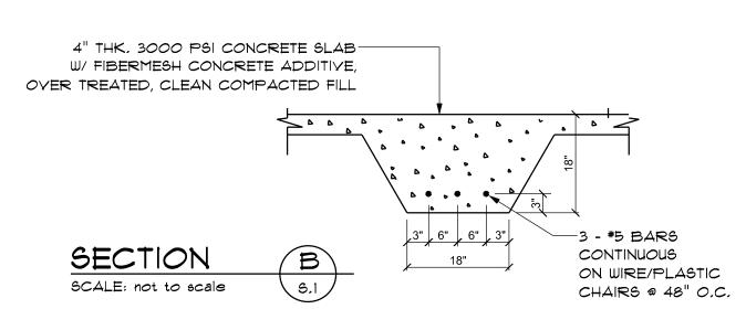
\* \* USE THIS DETAIL AT INTERIOR BEARING WALLS (SEE TRUSS CO., LAYOUT FOR POSSIBLE LOCATIONS) \* \*
