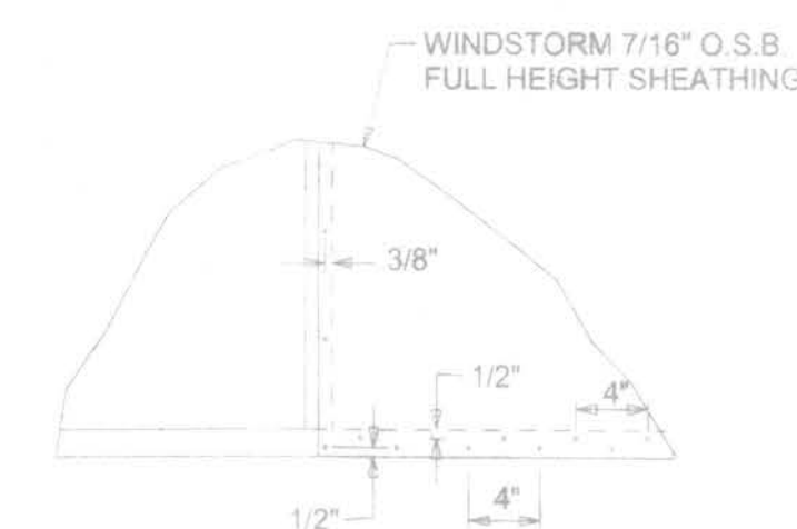
DOUBLE NAIL EDGE SPACING TOP AND BOTTOM PLATE UPLIFT CAPACITY = 474 plf (TABLE 305S1 SSTD10-99)
