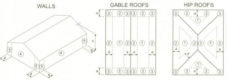
a: 10% of least horizontal dim. or 0.4h, whichever is smaller, but not less than either 4% of least horizontal dimension or 3 ft.
