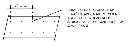
NAIL PLYWOOD FLITCH BEAM TOGETHER W/ 16d NAILS STAGGERED TOP AND BOTTOM, EACH FACE WHERE BEAM SPAN IS GREATER x - x -THAN 8'-0", CENTER 8'-0" LONG PLYWOOD AT CENTER OF BEAM SPAN, BUTT ADJACENT PLYWOOD PIECES TIGHT TO CENTER PIECE. STAGGER JOINTS AT BEAMS WITH MORE THAN ONE PLYWOOD PLATE.
