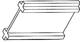
MEDIUM MULLION REINFORCEMENT #16990 ALUMINUM 6063-T6
