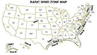
NOTE: See Section 3280.305(c) (2) for areas included in each Wind Zone SIGN ROOF LOAD ZONE MAP North 40 PSF XX South 20 PSF DESIGN ROOF LOAD ZONE MAP XX South 20 PSF
