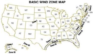
NOTE: See Section 3280.305(c) (2) for areas included in each Wind Zone DESIGN ROOF LOAD ZONE MÀP North 40 PSF XX South 20 PSF
