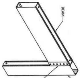
STANDARD BEAM TO U-CHANNEL CONNECTION (SHOWN FROM ISOMETRIC TOP)
