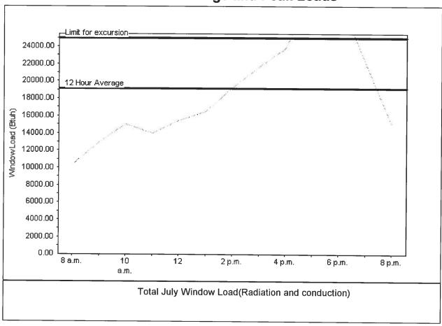
This application has glass areas that produce large heat gains for part of the day. Variable air volume devices are required to overcome spikes in solar gain for one or more rooms. Install a zoned system or provide zone control for problem rooms. Single speed equipment may not be suitable for the application.
