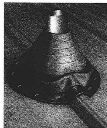
Figure 10 Pipe Boots provide a water-tight seal around roof vents and come in a variety of sizes. They seal with caulk and conform to the shape of the panel ribs.
